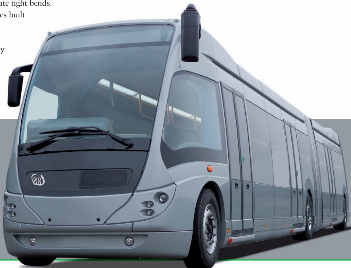
Reference project for the 2010 World Hydrogen Energy Conference in Essen: together with partners, Vossloh is developing for series production a fuel-cell bus running on hydrogen.
