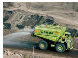
Once of Adaro's four mining contractors, Buma sprays an input haul road to keep dust down.
