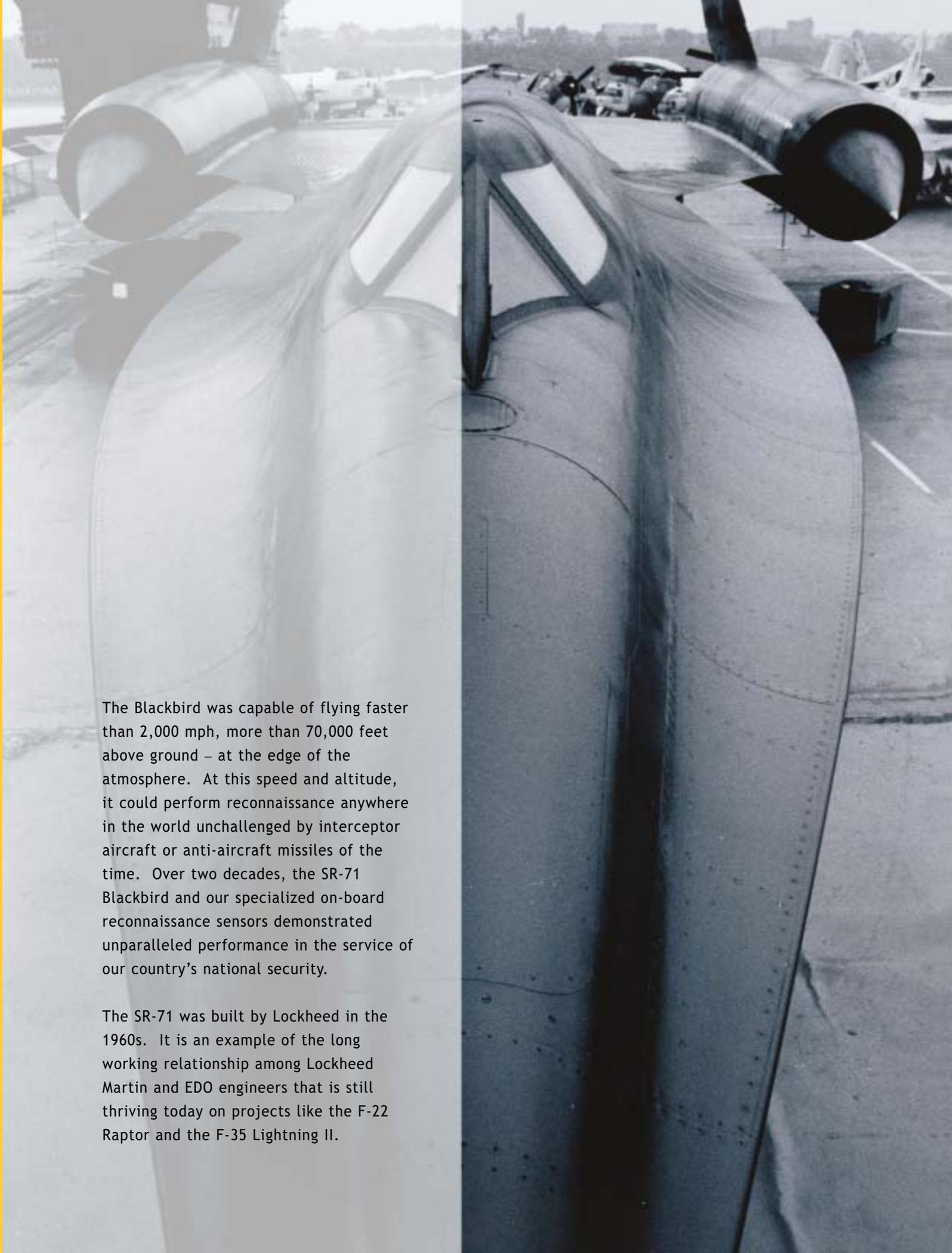
The Blackbird was capable of flying faster than 2,000 mph, more than 70,000 feet above ground – at the edge of the atmosphere. At this speed and altitude, it could perform reconnaissance anywhere in the world unchallenged by interceptor aircraft or anti-aircraft missiles of the time. Over two decades, the SR-71 Blackbird and our specialized on-board reconnaissance sensors demonstrated unparalleled performance in the service of our country's national security.
