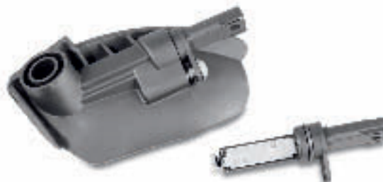
Heated blow-by pipe
