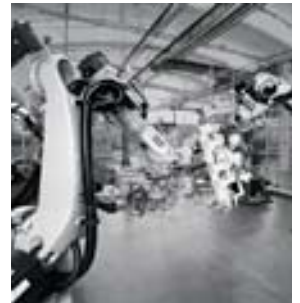
Jigless bodyshop with cooperating robots.
