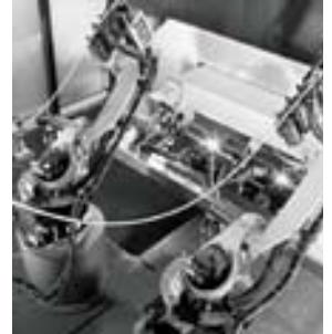
KUKA robots work hand-in-hand to weld a car body.
