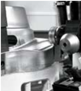
HOQ hemming – robot-based flanging with short cycle times.
