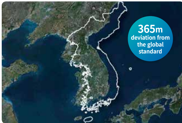
* Today, the location of Korea based on the Japanese origin (Tokyo Datum) deviates from the international standard by approximately 365m.
