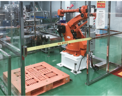
1 An improvement in working conditions: Using soundproof electronic earmuffs 2 An improvement in working conditions: Installing industrial robot protective fences
